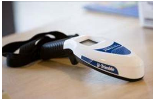
Fig 2. The hand held sensor use to obtain NDVI data at “ground” level.
