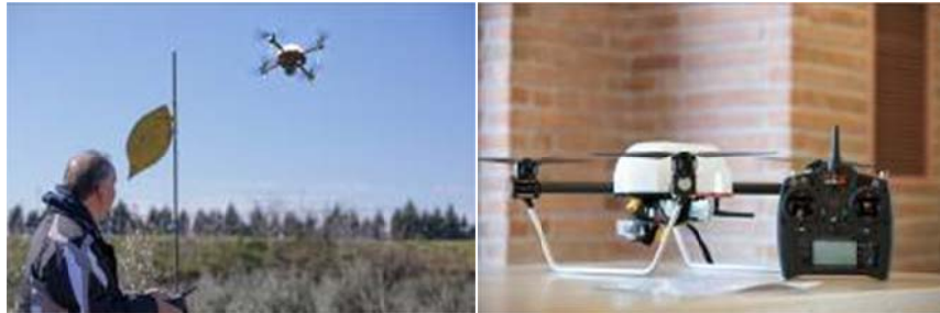
Fig 1. The UAV used for the study to obtain “aerial” NDVI data.
